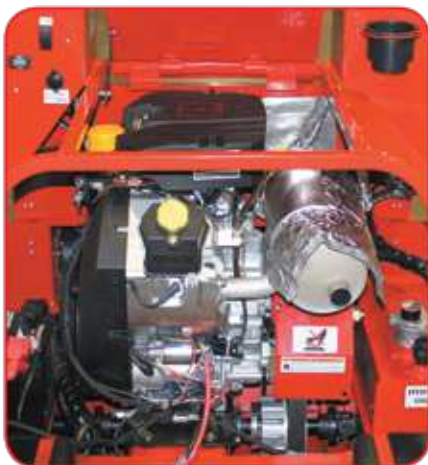
Powerful Kohler Air-Cooled Engine is easily accessible through the flip-up seat and removable front panel.
