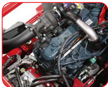
44HP Turbo-Charged Kubota Diesel Engine
